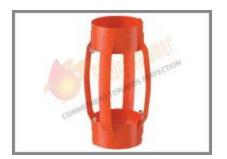
SledgeHammer's Welded Hinged Spring Bow Centralizers are high quality welded products, which meet or exceed API 10D specification. Welded Centralizer has more Restoring Force as compare to Non Welded Centralizer. The Centralizers have Bow Spring strongly welded to the End Collar under required temperature and condition with extra low Hydrogen coated Electrodes.
